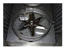
After drying inner layers are cooled down to approx. 82 F, (25°C). Room air is drawn in and led through a heater exchanger. The used cool air will be led to the exhaust air.
